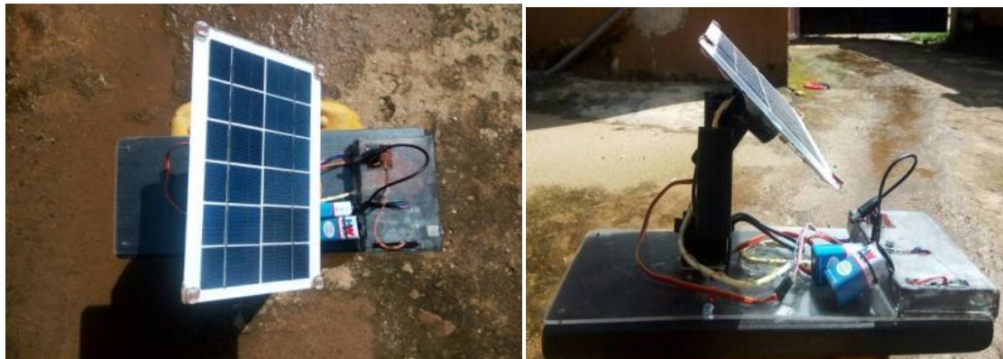
Plate 2: Constructed dual axis solar tracker
